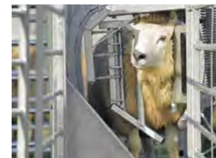
9. AUTOMATIC HEAD YOKE Unique feature fixing head in position when shoulders hit panel
