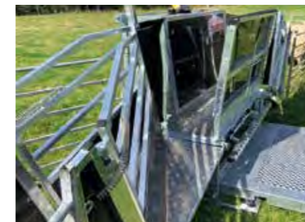
5. THREE WAY DRAFT Allows animal to exit in three directions into penning
