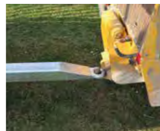
FIXED DRAWBAR WITH PICK-UP HITCH AND REMOVABLE STAND
