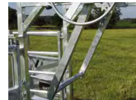
7. DROP DOWN RUMP BAR Ratchet style rump bar
