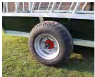
10.0 75 X 15.3 6-STUD WHEELS ON 60MM STUB AXLES
