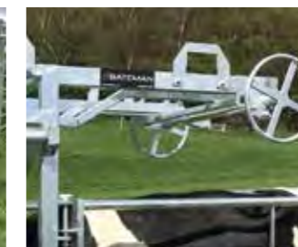
WHEEL-OPERATED FRONT DOORS
