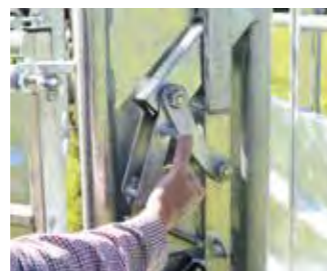
WIDTH ADJUSTMENT FOR YOKE
