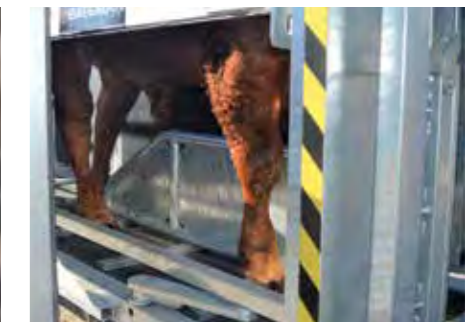
8. RUBBER FLOOR MATTING AND BRISKET RAIL For noise reduction with Brisket Rail to prevent animal 'going down'
