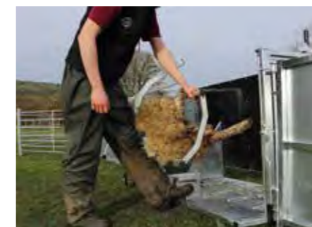
8. FOOT PEDAL Allowing cradle to be swung out for access all round the animal
