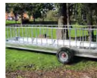
WELDED STEEL CHASSIS AND TROUGH, FULLY GALVANIZED
