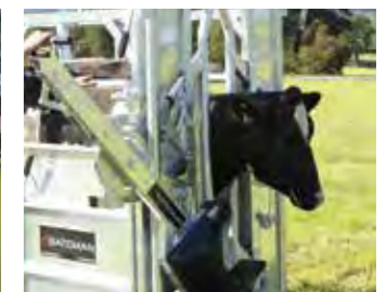
SWINGS OUT OF THE WAY TO ALLOW EASY RELEASE
